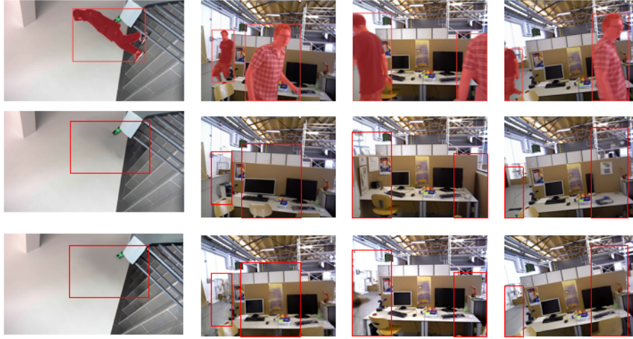
Fig. 1: Image showcases the ground truth of dynamic objects at the top, the inpainting of the image using LaMa [41] in the middle, and the inpainting using our method at the bottom. Our method removes moving objects and real inpaints scene details, such as laptops or posters.
