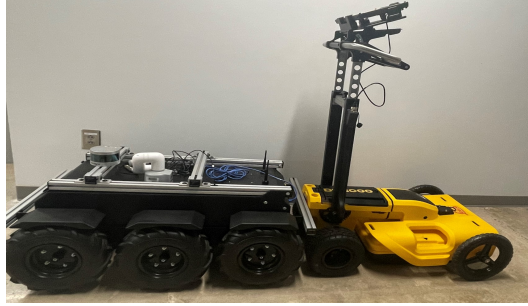
Fig. 2: Omnidirectional robot for GPR data collection, where the robot (HK1500) tows
