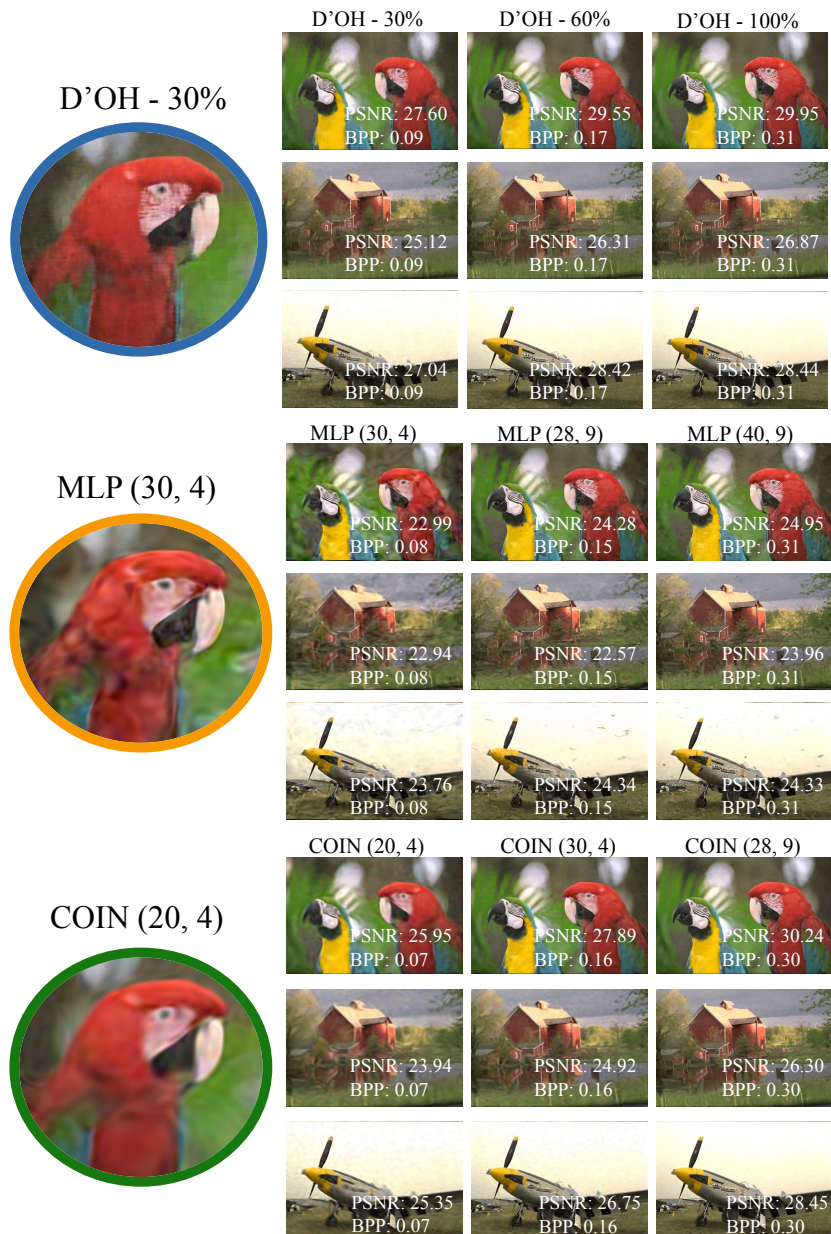
Fig. 7: Additional qualitative results on Kodak showing the comparison between 8-bit D'OH, 8-bit MLP, and COIN (a MLP quantized to 16-bits). Note that smaller COIN architectures are required to match the comparison bit-rates. D'OH is more robust to quantization than the MLP models. D'OH uses positional encoding, while the MLP models do not (see: Figure 3a) - PE is detrimental to low-rate MLP performance).
