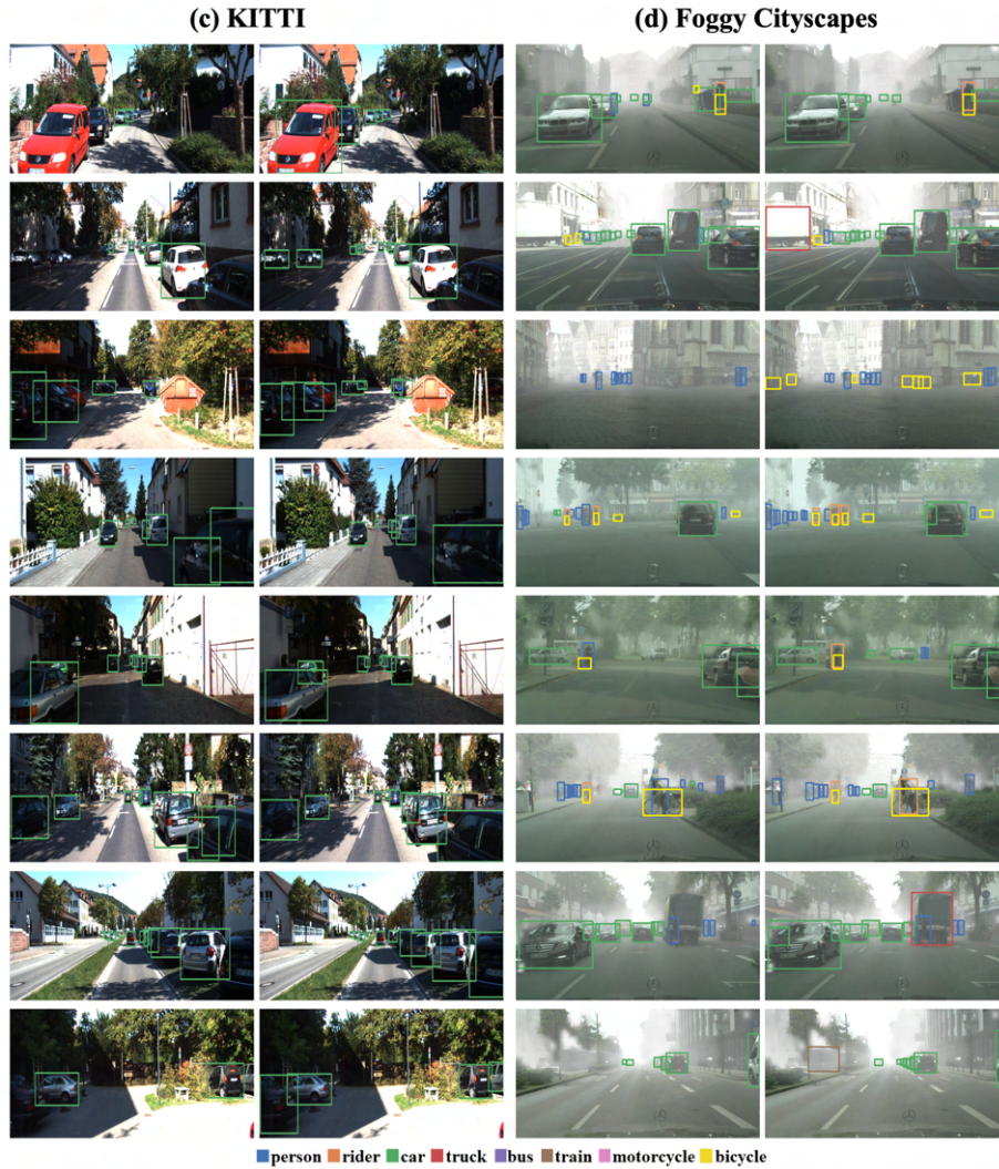
Fig. 9: Additional qualitative results employing our proposed DuPDA method are presented for (c) scene adaptation using the KITTI dataset and (d) weather adaptation using the Cityscapes dataset scenarios. The comparisons are displayed column-wise; from left to right: columns 1 and 3 depict the results of the SWDA baseline, while columns 2 and 4 show the results of our DuPDA.
