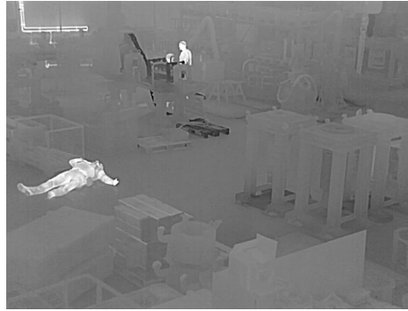
Fig. 1: Thermal image of a worker lying unconscious in a maintenance hall. Colleagues are not able to see him to call for help.
