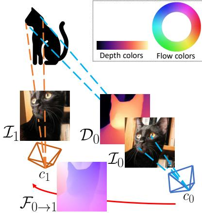
**Figure 2. Overview of the proposed depthstillation pipeline.** Given a single image  $\mathcal{I}_0$  and its estimated depth map  $\mathcal{D}_0$ , we place the camera in  $c_0$  and *virtually* move it (red arrow) towards a new viewpoint  $c_1$ . From the depth and virtual ego-motion, we obtain optical flow labels  $\mathcal{F}_{0 \rightarrow 1}$  and a novel  $\mathcal{I}_1$  through forward warping.
