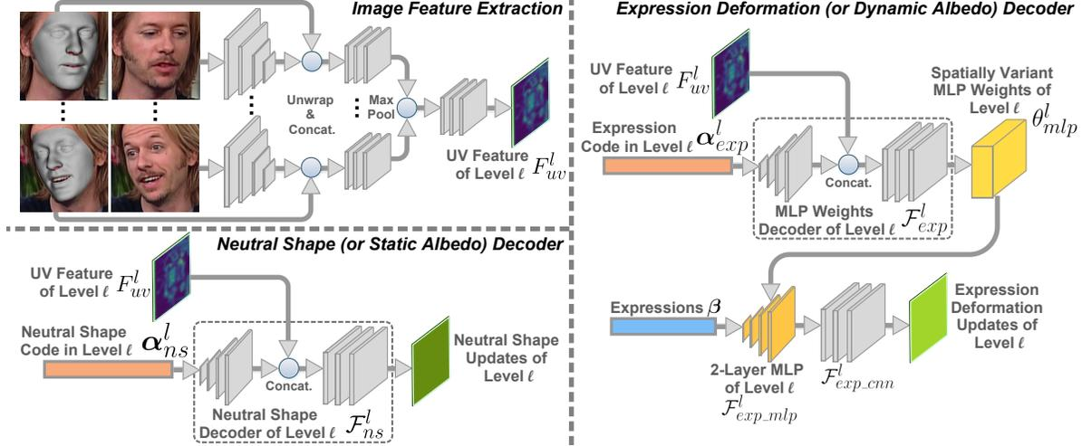
Figure 3. The illustration of different components in our neural rig decoder (Sec. 3.1). Top left: **Image Feature Extraction**. Bottom left: **Neutral Shape (or Static Albedo) Decoding**. Right: **Expression Deformation (or Dynamic Albedo) Decoding**.
