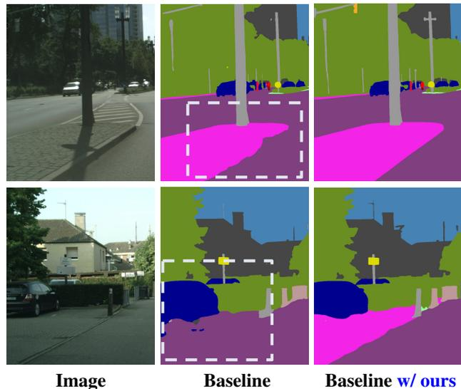
**Figure 1:** Left: Images from Cityscapes *val* benchmark [9]. Middle: Segmented prediction for an HRNet-48-OCR [45] [49] baseline. Right: Same backbone trained using our InverseForm boundary loss. Our model achieves clear improvements, e.g. the curbside boundary in the top figure is aligned better with the structure of boundary, and the curbside in the bottom is correctly detected.
