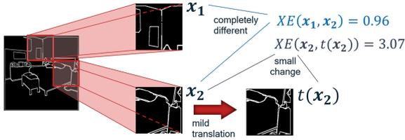
**Figure 2:** Cross-entropy(XE) based distance fails for spatial transformations of boundaries. In the above example,  $x_1$  and  $x_2$  are slices sampled from a boundary map. Only a mild shift is applied to  $x_2$  to generate a third slice  $t(x_2)$ .
