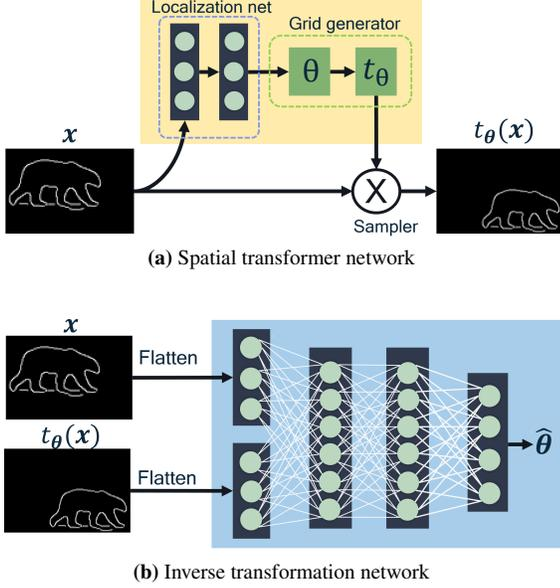
**Figure 3:** Spatial transformer (a) and our inverse-transformation network (b). Our inverse-transformation network architecture inputs two images  $x$  and  $t_\theta(x)$ , and predicts the transformation parameters  $\hat{\theta}$ . This performs the inverse operation as that of the spatial transformer network.
