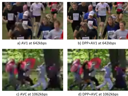
Figure 1: Left: Frame segments of encoder vs. DPP+encoder at the same bitrate. Right: Bjontegaard delta-rate vs. runtime (in multiples of x264 slow preset runtime on CPU) for codec only (red) and DPP+codec (green). More negative BD-rates correspond to higher average bitrate savings for the same visual quality. x264: AVC/H.264, aomenc: AV1, vrenc: VVC/H.266).
