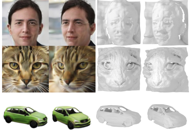
Figure 9: We can extract a proxy 3D representation as a mesh, either by projecting a depth-map (CelebA, Cats), or through marching cubes (CARLA).
