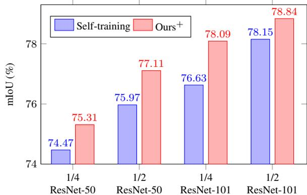
Figure 5: **Comparison with self-training** on PASCAL VOC 2012. The self-training approach is a two-stage approach which takes more training epochs. For a fair comparison, we train our approach with more training epochs (denoted by ‘Ours<sup>+</sup>’) so that their epochs are comparable. The CutMix augmentation is not used.
