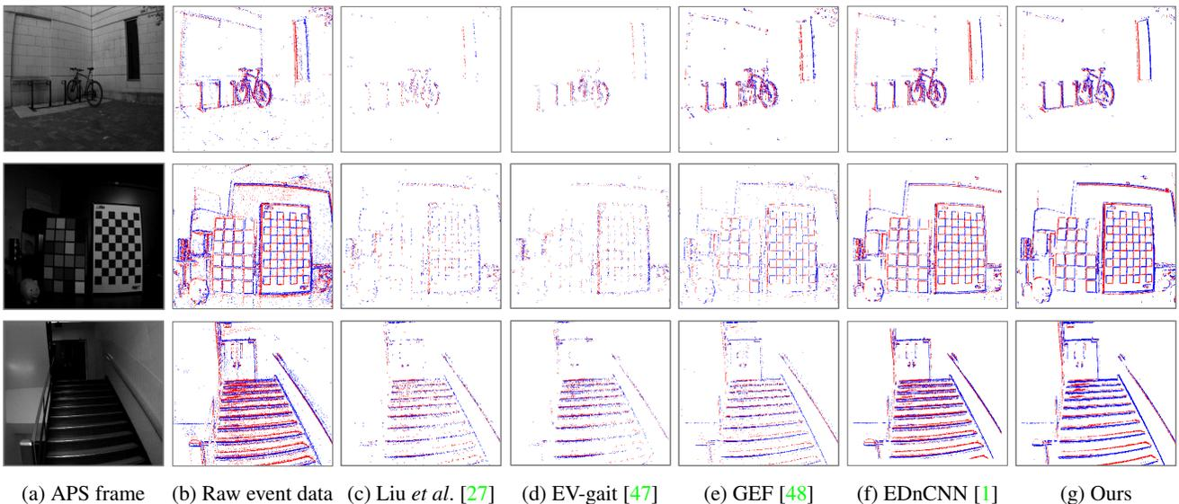
Figure 5: Same-resolution denoising results on the DVSNOISE20 [1] dataset. (a) an APS frame captured by a DAVIS346. (b) the event frame accumulating events fired within the exposure time of (a). (c)-(g) the denoising results based on (b).
