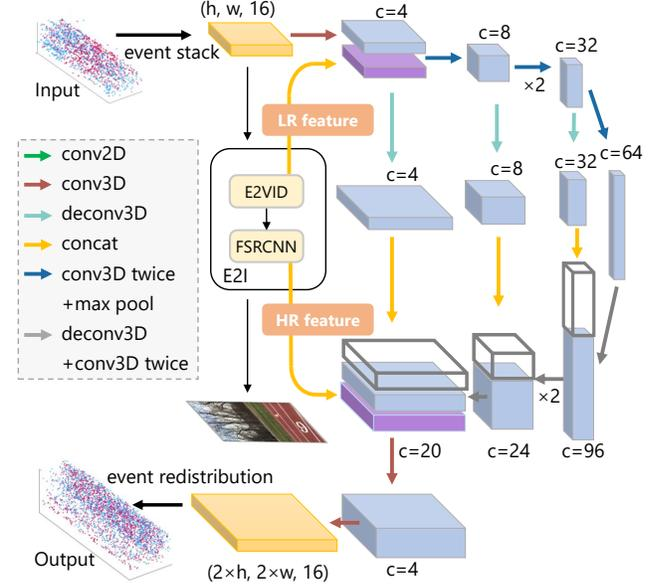
Figure 4: EventZoom- $2\times$  network architecture. The input LR events are first binned into a 16-channel event stack. The event stack is then fed into two branches, *i.e.* a 3D U-Net and an E2I module which consists of E2VID [36] and FSRCNN [9]. The LR and HR features from the last layer of E2VID and FSRCNN are concatenated with the beginning and second last layers of the U-Net. Finally, the HR event stack is redistributed to spatiotemporal point clouds.
