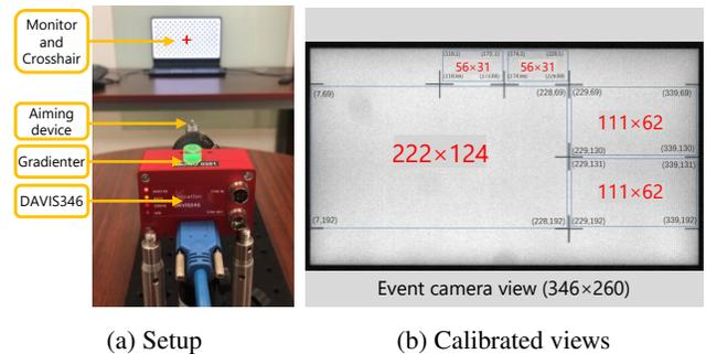
Figure 2: We implemented a display-camera system to study event formation and degradation. The display has been divided into 5 segments with two  $1\times$ , two  $2\times$  and one  $4\times$  resolution scales.
