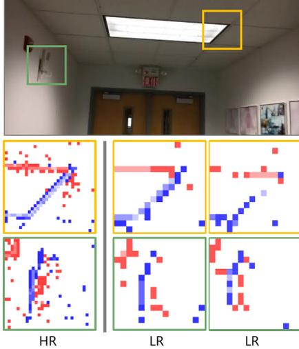
Figure 3: Visualization of an NFS [14] video frame (upper panel), recorded events for the HR video (lower left), and two repeated event recordings of the  $2\times$  downsized LR video (lower middle & right).
