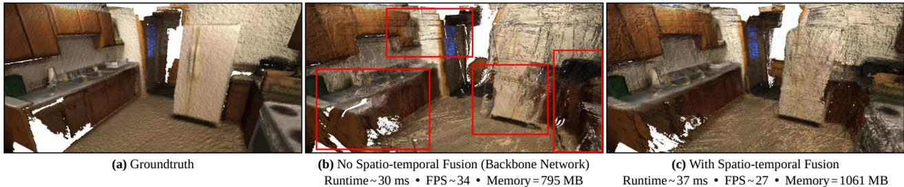
**Figure 1:** 3D reconstructions of a scene from ScanNet [11]. Extending our stereo backbone with our proposed spatio-temporal fusion module improves the temporal consistency and accuracy of the predicted depth maps, leading to better reconstructions with negligible computational overhead. Runtime is per forward pass on an NVIDIA GTX 1080Ti with image size  $320 \times 256$ .
