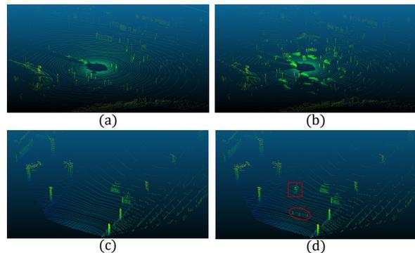
**Figure 1:** Examples of augmented LiDAR data, where (a), (c) are the original LiDAR point cloud and (b), (d) are the augmented LiDAR point cloud by “LiDAR-Aug”. Specifically, the “LiDAR-Aug” can be used to expand the rare objects such as traffic cone and cyclist which has been highlighted in the sub-fig (d).
