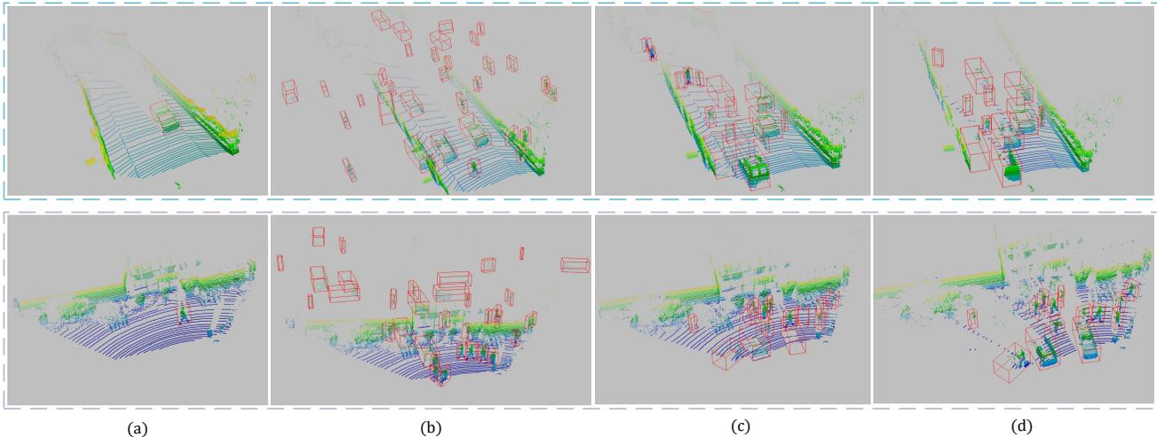
**Figure 5:** Visualization comparison between “GT-Aug” and “LiDAR-Aug”. (a) shows the original data with annotation from KITTI; (b) shows the augmented LiDAR data with “GT-Aug”; (c) shows the augmented LiDAR data with “GT-Aug” but the poses are sampled with ValidMap; (d) shows the augmented LiDAR data with “LiDAR-Aug” while the poses keep the same as in (c).
