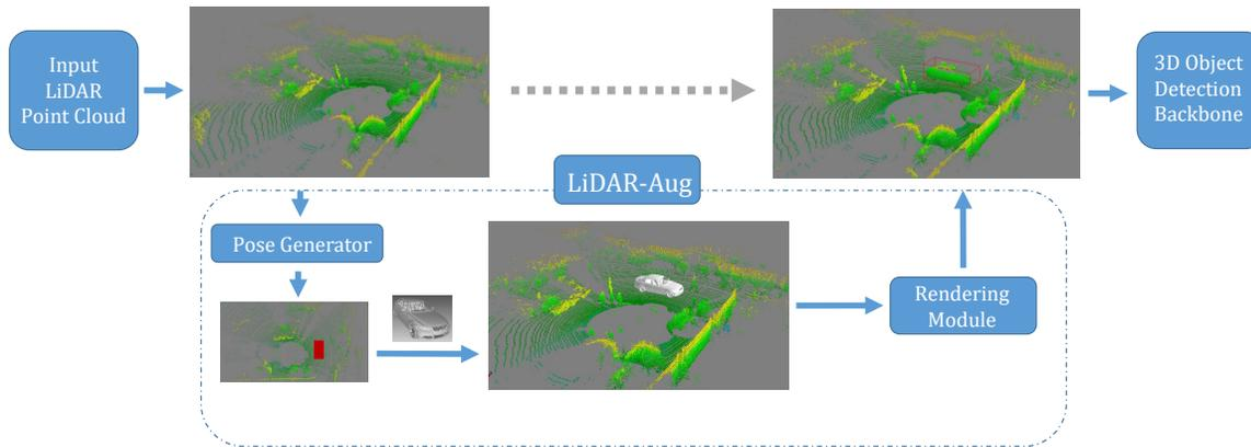
**Figure 2:** The overview of our proposed “LiDAR-Aug” framework. The input original LiDAR point cloud is first sent to the “Pose Generator” module. Then the CAD models are inserted into the scene under the sampled poses, after which the augmented LiDAR point cloud is generated by rendering the inserted models onto the original background via the “Rendering Module”. We then exploit the augmented LiDAR data and validate the effectiveness in the 3D object detection task.
