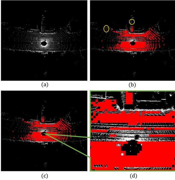
**Figure 3:** Pose generator with ValidMap. (a) Original input LiDAR point cloud with bird’s-eye-view; (b) ValidMap shown in red color pixels are overlaid with (a); (c) Post-processing results for the ValidMap with the isolated pixels marked by yellow circles in (b) are removed; (d) better illustration for (c) by zooming in.
