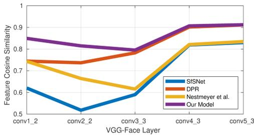
Figure 8: **Facial Detail Preservation on Multi-PIE.** We compute the cosine similarity between the VGG-Face [21] features of each method’s relit images and groundtruth target images to measure their ability to preserve local and global facial details during relighting. Our method is consistently the best at preserving local details based on the cosine similarity in the *earlier* layers.
