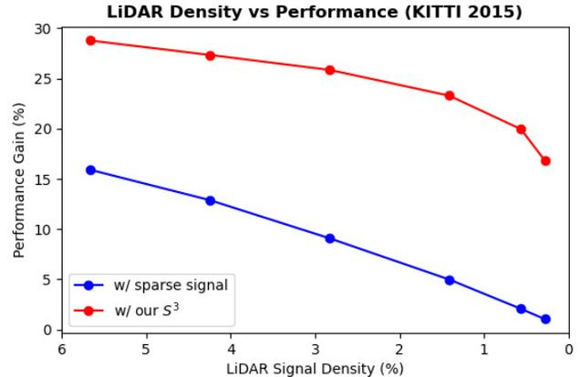
Figure 6: **Density vs Performance.** The figure stresses the robustness of  $S^3$  for extremely low signal density.
