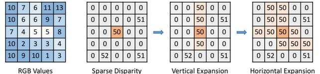
Figure 3: **Intuition for sparse signal expansion by ad-hoc method.** Sparse depth map (right) is expanded according to RGB image (left) presented in one channel here. Zero in the sparse map means no signal. The example expands the center signal according to difference of color intensity with threshold = 2.
