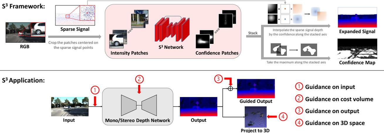
Figure 2: **Sparse Signal Superdensity ( $S^3$ ) overview.** The top pipeline illustrates the details of  $S^3$  framework to expand sparse signal and generate the final expanded depth and confidence map (Section 3.2). The bottom demonstrates the application of our module to guide on different stages of depth estimation (Section 4).
