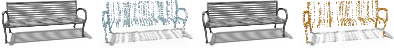
Figure 3: Two point clouds with 3K points drawn with the BNL [33] quasi-random sequence for two different triangulations describing the same 3D model. One would expect to have a very close distance between the point clouds, however, due to the deterministic nature of the sampler, some artefactual patterns appear.
