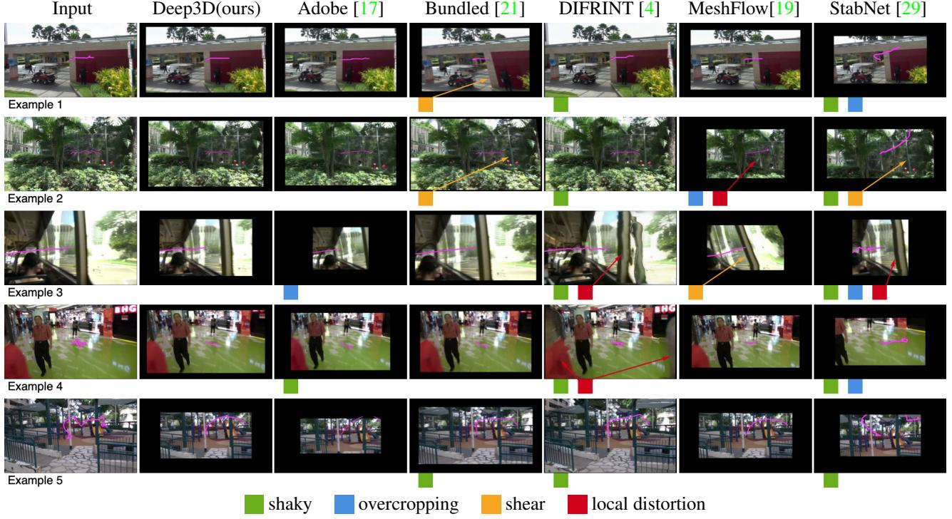
**Figure 7. Visual comparison of the state-of-the-art methods:** The artifacts are noted below thumbnails. The magenta paths on the thumbnails indicate the optical flow motion of the resulted videos. Smoother paths represent the more steady results. To visualize the cropping loss of each result, we rescale each video to the input scale. The distortion and shear are pointed out by yellow and red arrows, respectively. Zoom in for a better (more detailed) visualization.
