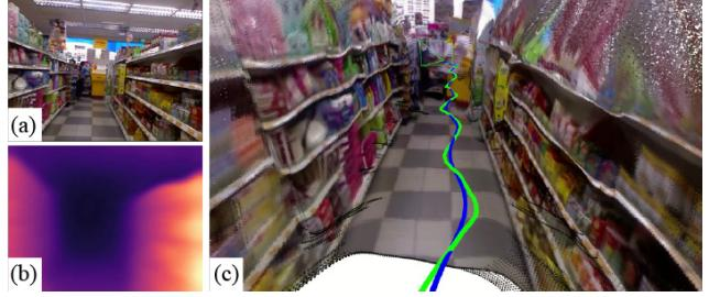
**Figure 5. Example of camera trajectory smoothing:** (a) Input video. (b) Depth  $D^*$  of (a). (c) The 3D model of the input video reconstructed by  $\{D_t^*, P_t^*\}_{t=1}^N$ . The green/blue paths represent the original/smoothed camera trajectories in 3D model, respectively.
