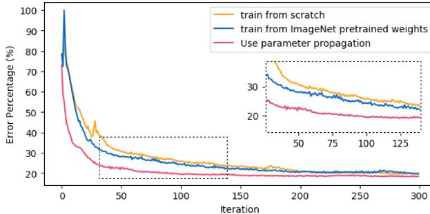
**Figure 4. Convergence speeds comparison:** The convergence curves averaged on all snippets (except for the first snippet) are shown for different parameter initialization strategies. Among them, parameter propagation shows the fastest convergence speed compared to training from scratch and ImageNet [26] pre-trained weights, which increases the test-time training speed better.
