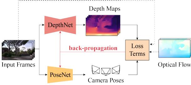
**Figure 2. 3D geometry optimization framework:** The DepthNet and PoseNet estimate dense scene depth and camera pose trajectory based on a snippet of the input sequence. The loss terms measured via 3D reprojection are used to update the parameters of DepthNet and PoseNet via back-propagation in test-time.
