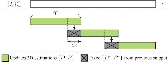
**Figure 3. Illustration of overlapping snippets:** An input sequence  $\{I_t\}_{t=1}^N$  is sequentially divided into length- $T$  snippets with  $\Omega$  frames overlap. For a current snippet (except for the first one), the 3D depth and pose estimations of the overlapping area (gray with  $\times$ ) are frozen as the optimal  $\{D^*, P^*\}$  estimated for the previous snippet. The learning framework only updates the non-overlapping  $\{D, P\}$  (green) to enforce the temporal coherence.
