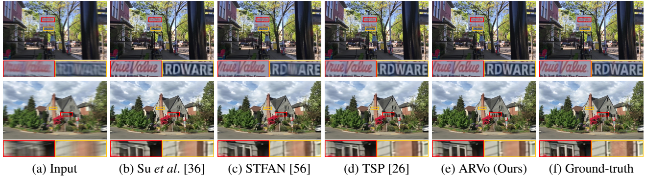
Figure 5: Qualitative comparisons on the DVD [36] dataset. Our model benefits from constructing pixel pair correspondence in the feature space, thus being able to better utilize neighboring sharp patches to improve the restoration quality.
