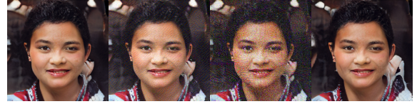
Figure 7. From left to right: reference image, image generated by FGSM L_{inf} , PGD L_{inf} and proposed method, all three adversarial images can deceive the detector. Zoom in to see more details.
