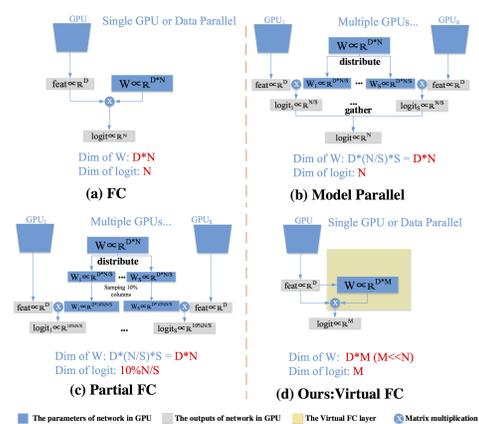
Figure 1. Comparison between FC (a), Model Parallel (b), Partial FC (c), and our Virtual FC (d).  $D$  is the dimension of features,  $N$  is the number of identities (categories),  $S$  is the number of GPUs, and  $M$  is a hyperparameter that can be set freely based on the balance between performance and computational resources.  $M = 1\% \times N$  in this paper.
