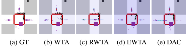
Figure 4: The figure illustrates predicted hypotheses and learned mixture distribution of goals using different WTA objectives on the CPI test set. The purple and black box represent car and pedestrian at their current location. Predicted hypotheses are shown in their respective colours. (e) captures the data distribution better with hypothesis spread out across the crosswalk resembling the ground truth distribution of points.
