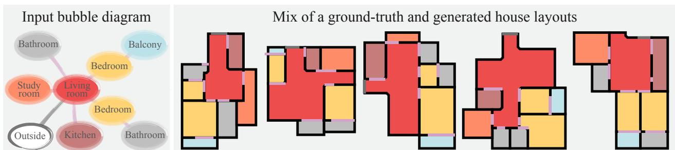
Figure 1. The paper makes a breakthrough in automated house layout generation. The right is the mix of a ground-truth design by an architect and our generated samples, based on the input bubble-diagram. (The second from the right is the ground-truth.) A novel generative adversarial layout refinement network is trained to repeatedly apply and refine the design towards perfection.
