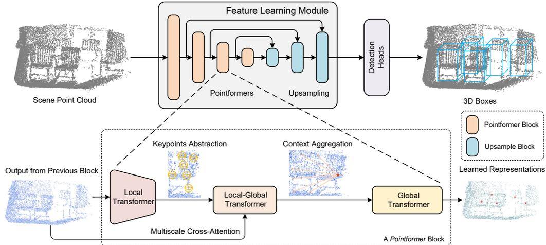
Figure 2. The **Pointformer** backbone for 3D object detection in point clouds. A basic feature learning block consists of three parts: a Local Transformer to model interactions in the local region; a Local-Global Transformer to integrate local features with global information; a Global Transformer to capture context-aware representations at the scene level.
