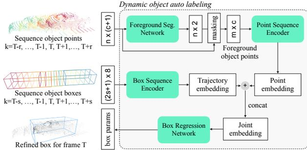
Figure 5. **The dynamic object auto labeling model.** Taking a sequence of object points and a sequence of object boxes, the model runs in a sliding window fashion and outputs a refined 3D box for the center frame. Input point and box colors represent frames.
