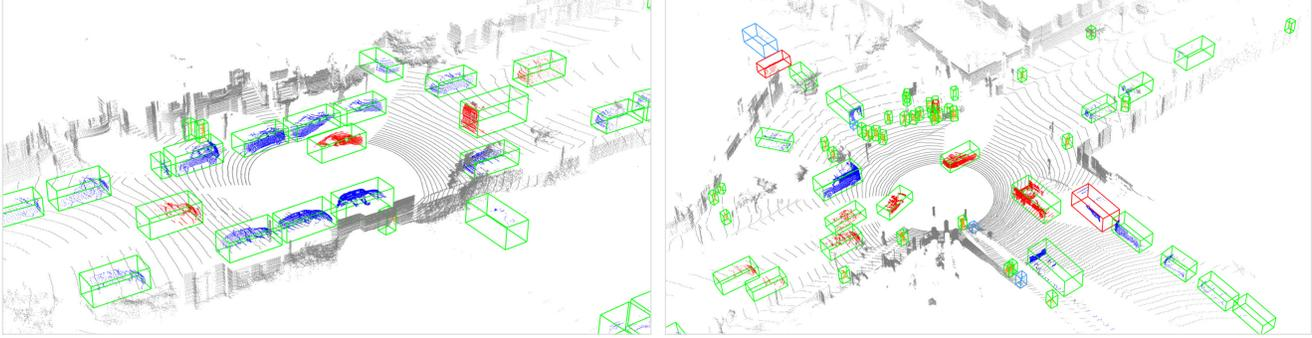
Figure 6. **Visualization of 3D auto labels on the Waymo Open Dataset *val* set** (best viewed in color with zoom in). Object points are colored by object types with **blue** for static vehicles, **red** for moving vehicles and **orange** for pedestrians. Boxes are colored as: **green** for true positive detections, **red** for false positives and **cyan** for ground truth boxes in the cases of false negatives.
