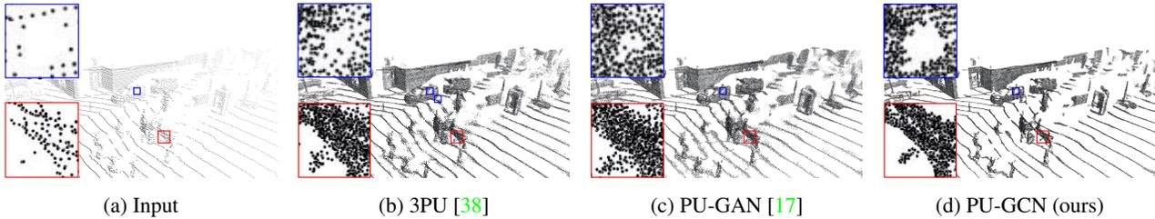
Figure 6: **Upsampling real-scanned point clouds from KITTI [7]**. PU-GCN preserves intricate structures and generates fine-grained details (e.g. the window of the car, the pedal of the motorcycle, etc.). Please zoom in to see details.
