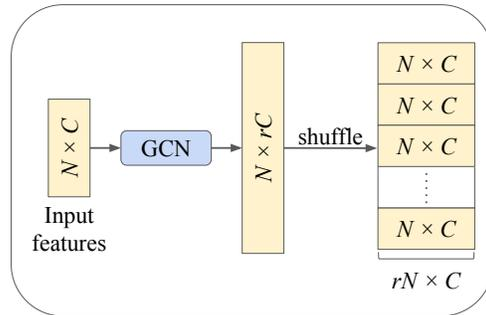
Figure 2: **Upsampling module: NodeShuffle.** We expand the number of input features by  $r$  times using a GCN layer, and then apply a shuffle operation to rearrange the feature map.  $r$  denotes the upsampling ratio.
