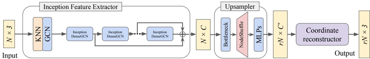
Figure 4: **PU-GCN architecture.** PU-GCN uses an inception feature extractor consisting of one or more Inception DenseGCN blocks, followed by the NodeShuffle based upsampler, and a coordinate reconstructor.
