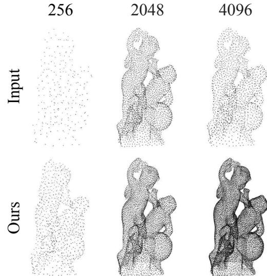
Figure 8: **Effect of input size.** The top row shows the input point clouds of different sizes, and the bottom row shows the  $\times 4$  upsampled outputs of our PU-GCN. PU-GCN always produces high quality results regardless of input size.
