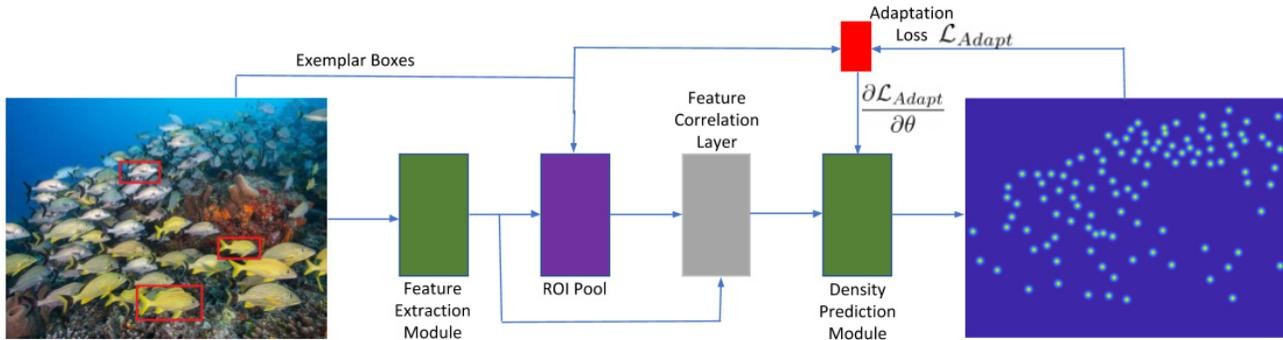
Figure 2: **Few-shot adaptation & matching Network** takes as input the query image along with few bounding boxes depicting the object of interest, and predicts the density map. The count is obtained by summing all the pixel values in the density map. The adaptation loss is computed based on the bounding box information, and the gradients from this loss are used to update the parameters of the density prediction module. The adaptation loss is only used during test time.
