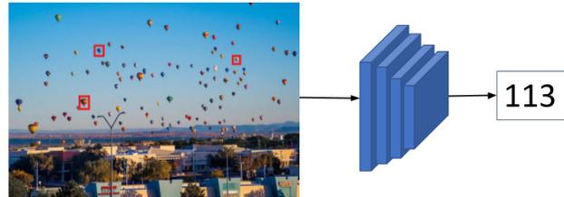
Figure 1: **Few-shot counting—the objective of our work.** Given an image from a novel class and a few exemplar objects from the same image delineated by bounding boxes, the objective is to count the total number of objects of the novel class in the image.
