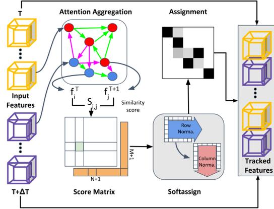
**Figure 3:** The learnable tracking framework. The input is the tesseract features for multiple detected humans at two different time instances. The output is an assignment matrix providing the correspondence between the detected persons at different times.
