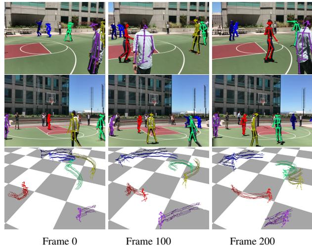
**Figure 1:** We illustrate the output of TesseTrack on the Tagging sequence. The top two rows portray the projections of keypoints on two views, while the bottom row shows the 3D pose tracking. Observe smooth tracking of people in the wild with moving cameras for long duration of time.
