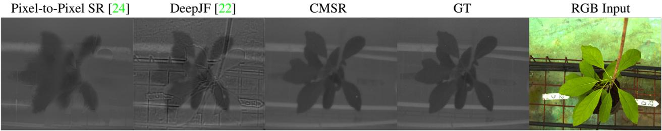
Figure 1: In this **visual-thermal** pair, the two inputs are displaced (visualised in Figure 6), a phenomenon which often occurs in real-world scenarios. This is a failure case even for state-of-the-arts, as they are based on perfect alignment. CMSR adapts to the given misalignment, and corrects it as a part of the SR process, producing a sharp result (41.069 dB PSNR). The deformed RGB image is presented in Figure 6
