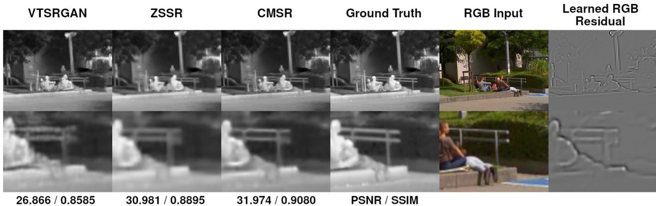
Figure 7: We compare our method to its baseline method, ZSSR ([6]), as well as to another cross-modality method, VTSRGAN ([1]) on a **visual-thermal** pair from the ULB17-VT evaluation. On the right, the output of *Feature-Extractor 2* (Figure 2) is given as the learned RGB residual which is added to our output. This RGB residual resembles an edge-map; it is artifact-free and contains no unwanted textures
