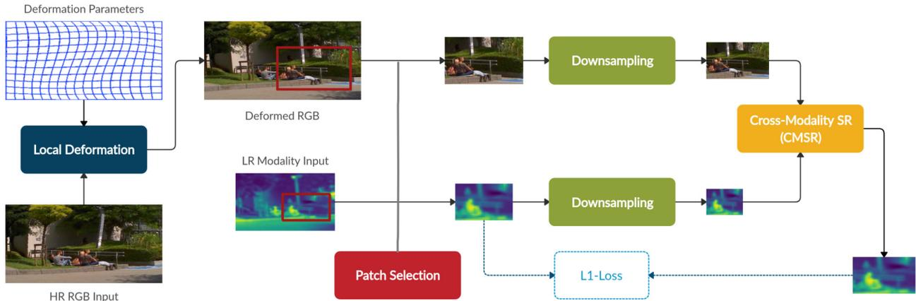
Figure 3: *Training process.* The RGB image first goes through a deformation step which aligns it to the target modality (in blue). Then, random patches are selected by an augmentation step (in Red) and down-sampled (in green). The patches are used to train the CMSR network (in orange) and the deformation parameters. The loss function is measured between the super-resolved output and the input target modality images.
