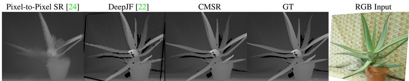
Figure 8: This misaligned **visual-depth** pair is taken from our *Shuffled*-Middlebury dataset evaluation. Compared to cross-modality state-of-the-arts, who struggle to produce a clear result, our method succeeds in this task (32.239 dB PSNR / 0.9403 SSIM) thanks to its alignment capabilities.
