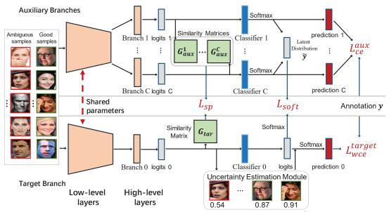
Figure 2: Overview of the DMUE. y denotes the set of annotations of images in a batch.  $\tilde{y}$  denotes the set of mined latent distributions of images in a batch.
