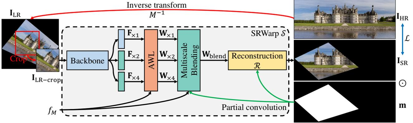
Figure 4: **Overall organization of the proposed SRWarp model.** More detailed architectures are described in our supplementary material. Black regions outside the warped image  $\mathbf{I}_{\text{SR}}$  represent void pixels that are ignored.
