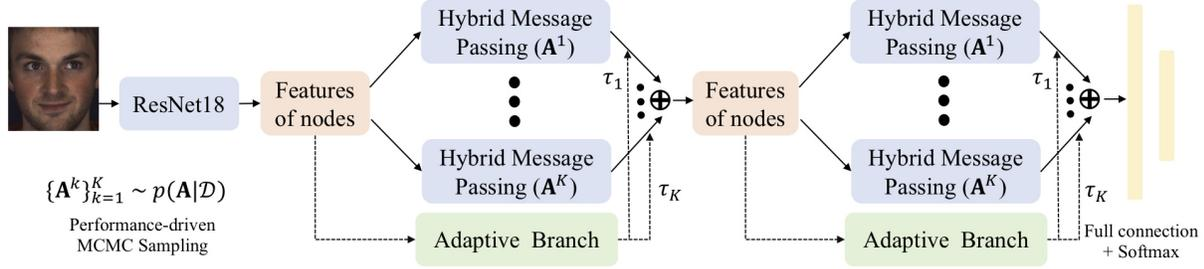
Figure 2. The architecture of hybrid message passing neural network with performance-driven structures for Facial AU detection. ResNet18 is the backbone network.  $\mathbf{A}^1, \dots, \mathbf{A}^K$  denote different graph structures generated by performance-driven MCMC sampling.
