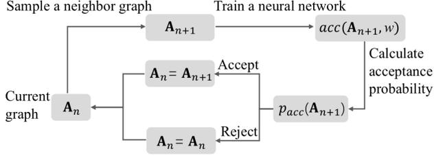
Figure 3. The framework of performance-driven MCMC sampling method to generate the graph structures.
