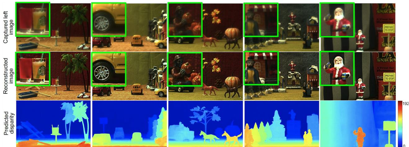
Figure 9. **Experiment results of various real-world scenes using our CodedStereo prototype.** Reconstruction results are shown for real scenes with both uniform background and non-uniform background (the last column, variation in texture/depth).
