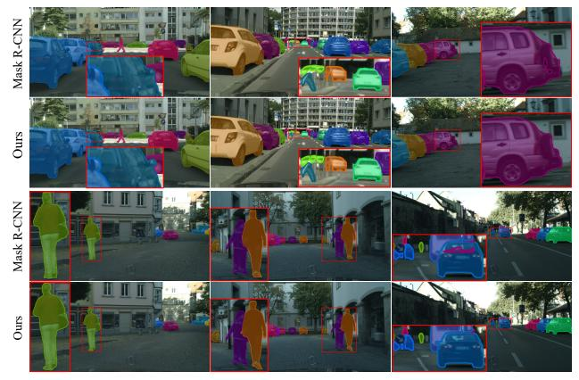
Figure 4: Qualitative results on Cityscapes val. The proposed framework (2nd and 4th rows) produces substantially better masks with more precise boundaries than Mask R-CNN (1st and 3rd rows). Best viewed digitally and in colour.
