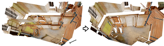
Figure 4. Example Sim3 registration, the network takes two RGB-D scans as input and predicts a similarity transformation which aligns the two scans.
