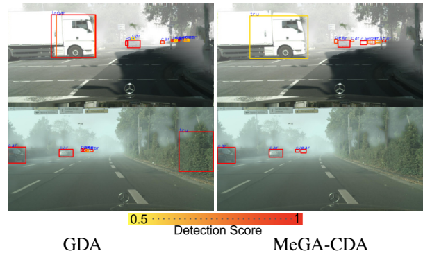
Figure 5. Qualitative detection results. Global alignment results in miss-detections. In contrast, the proposed approach reduces false-positives while achieving high-quality detections.
