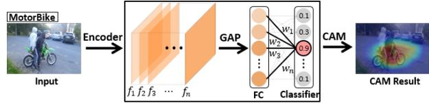
Figure 3. Illustration of the class activation mapping (CAM) details. FC: fully connected layer; GAP: global average pooling; numbers in the classifier represent the classification confidences.
