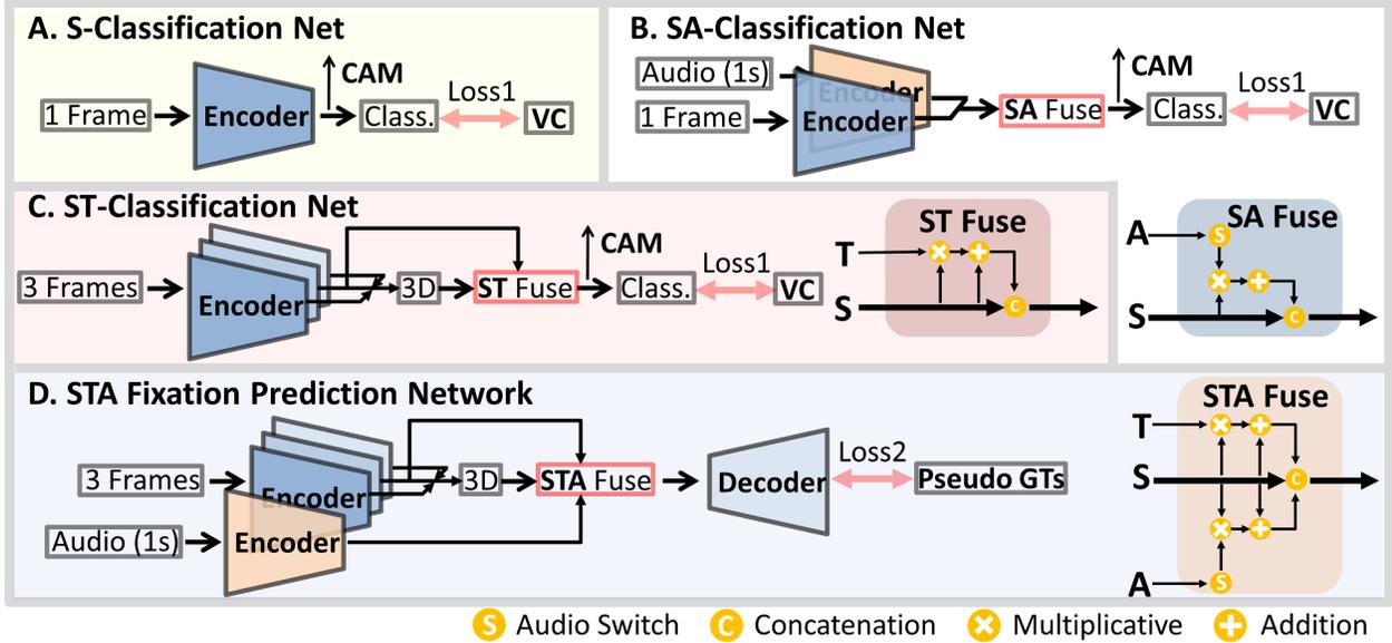
Figure 6. Network Details. Loss1: cross entropy loss; Loss2: binary cross entropy loss; ‘Class.’: Classification; VC: Video Categories; Decoder: VGG16; ‘3D’: 3D convolutional; A-C respectively show the network architectures of the adopted classification nets (Fig. 4); D is the STA fixation prediction network.
