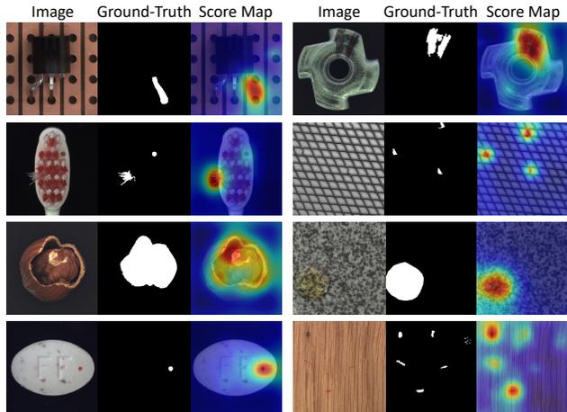
Figure 3. Qualitative anomaly localization results on MVTec AD dataset [6]. For each example, the images from left to right are the defective image, the ground-truth, and the anomaly score map produced by our algorithm. Zoom in for details.
