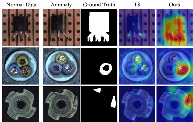
Figure 4. Qualitative comparisons on MVTEC AD dataset [6] between TS [7], which considers only local patches for anomaly localization, and our approach. Through adequately utilizing both the global and the local information, we manage to identify the transistor shift (first row), the cable swap (second row), and metal nut bend (third row) anomalies that are omitted by TS.
