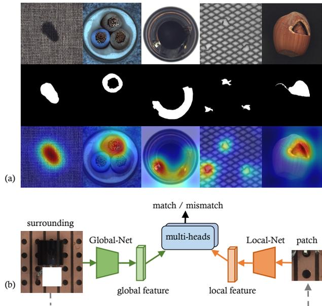
Figure 1. (a) **Anomaly localization results** where our approach can precisely segment the anomalous regions. From top to bottom: abnormal samples, ground-truth, and anomaly score maps produced by our algorithm. (b) **Concept diagram of global and local feature comparison.** Local-Net and Global-Net are employed to extract features from a patch and its surrounding respectively. Multiple anomaly detection heads are designed to determine whether the global and local features match or not.
