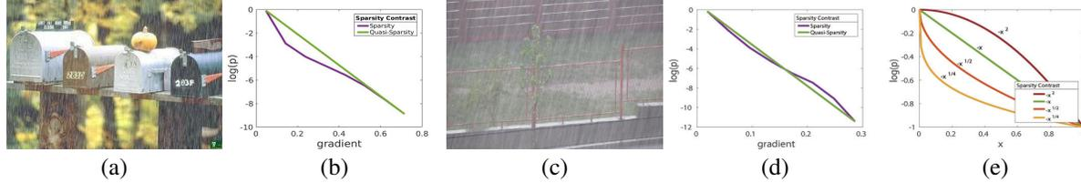
Figure 2. (a) Rainy image. (b) Log-histogram after (a) is filtered. (c) Non-sparse rainy image. (d) Log-histogram after (c) is filtered. (e) Log-probability of some stochastic distributions. According to [13], Gaussian distribution is non-sparse as it is above the straight line. Laplace distribution results in the straight line, which is the demarcation line of sparsity and non-sparsity.
