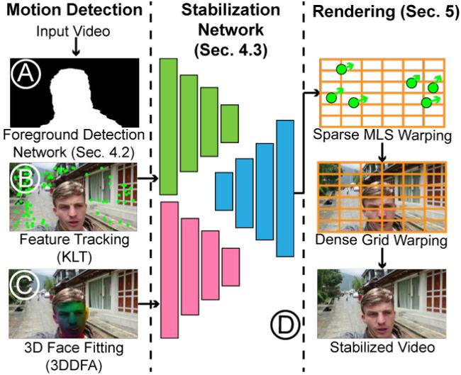
Figure 2. *The pipeline of our method.* (A) We first detect the foreground regions of the input video frame. (B) The background motion is tracked using feature points. (C) The foreground motion is tracked using 3D face vertices. (D) We train a stabilization network to infer the displacement of the MLS warp nodes. Finally, we use a grid to approximate the MLS warping and generate the stabilized frame.
