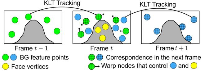
Figure 3. *The warping strategy of our method.* The background feature points in the same color are in correspondence. The feature points with grid patterns are the warp nodes. The arrows represent the MLS warping operation. During the stabilization, both the feature points  $P_t$  (solid blue points) and the face vertices  $F_t$  (solid yellow points) are warped by the warp nodes  $Q_t$  (grid green points).
