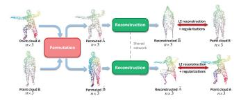
Figure 1. Illustration of the motivation of our unsupervised deep learning-based framework for computing dense correspondence between two point clouds.
