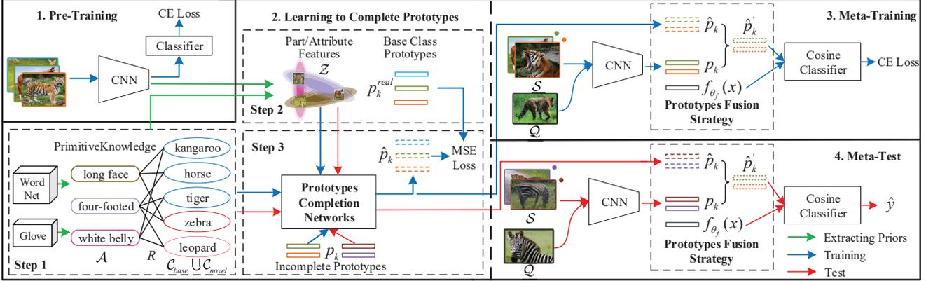
Figure 2. The prototype completion based meta-learning framework.
