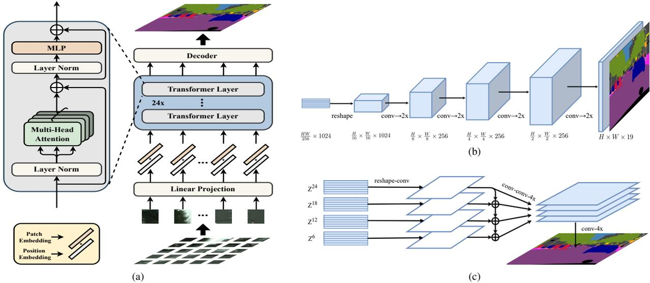
Figure 1. **Schematic illustration of the proposed *SEgmentation TRansformer (SETR)*** (a). We first split an image into fixed-size patches, linearly embed each of them, add position embeddings, and feed the resulting sequence of vectors to a standard Transformer encoder. To perform pixel-wise segmentation, we introduce different decoder designs: (b) progressive upsampling (resulting in a variant called *SETR-PUP*); and (c) multi-level feature aggregation (a variant called *SETR-MLA*).
