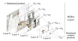
Figure 2: An illustration of MPI representation.
