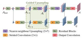
Figure 5: The multiscale guided upsampling module gradually enriches details of the initial alpha maps by introducing multiscale guidance from the reference view. For the operation of each level as depicted in the dashed green box, please refer to Eq. (3).
