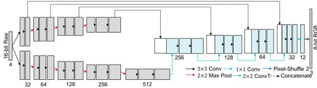
Figure 5: Network structure of the proposed UNet. It takes a 4-channel RAW sensor data observation  $y$ , and outputs the restored 3-channel RGB image  $x$ .
