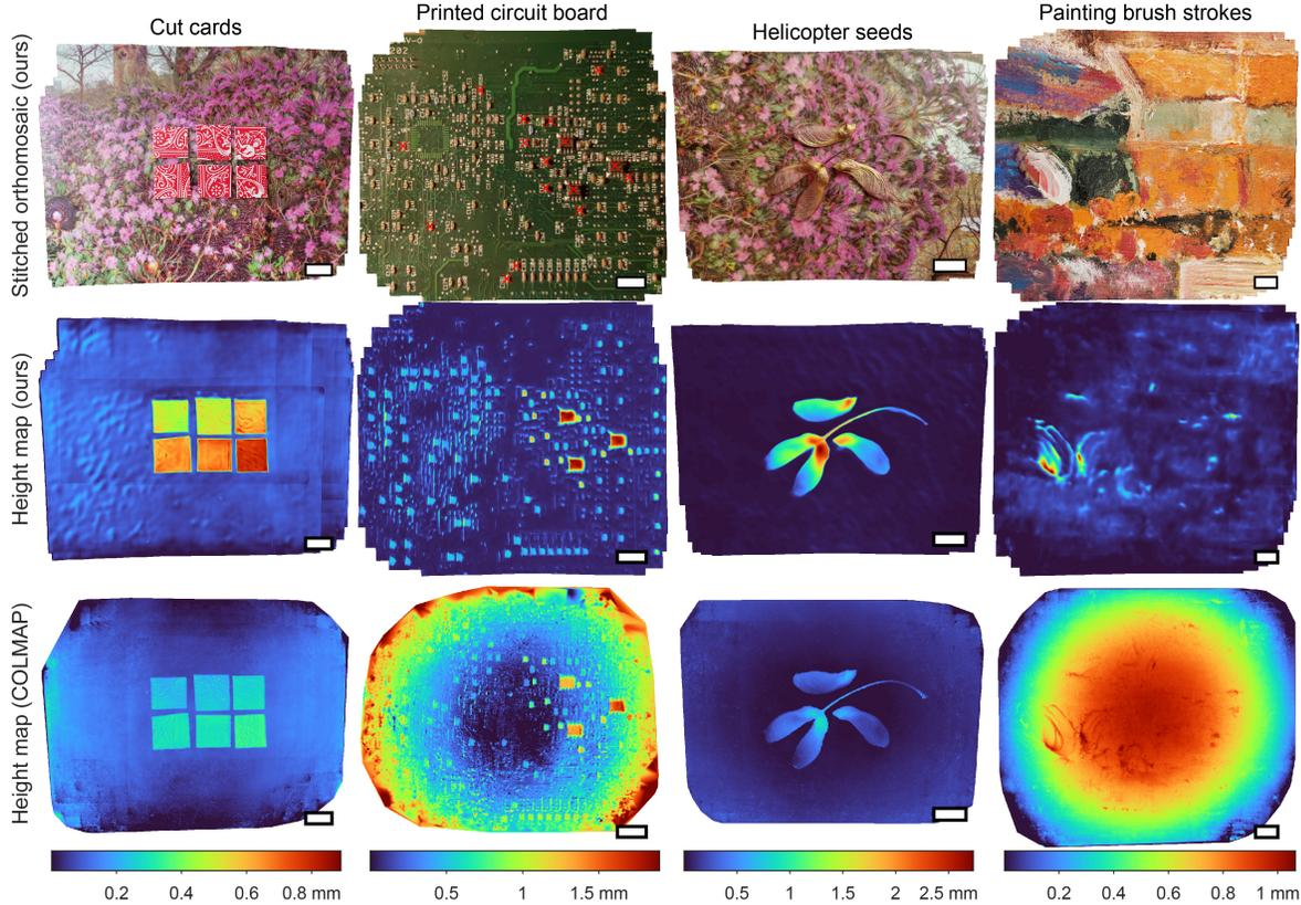
Figure 4. Stitched orthomosaics and height maps for various samples with mm-scale height variation. Height values for the cut cards and PCB components (red  $\times$ 's) are quantified in Tables 1 and 2, respectively. COLMAP consistently underestimates heights. Scale bars, 1 cm.
