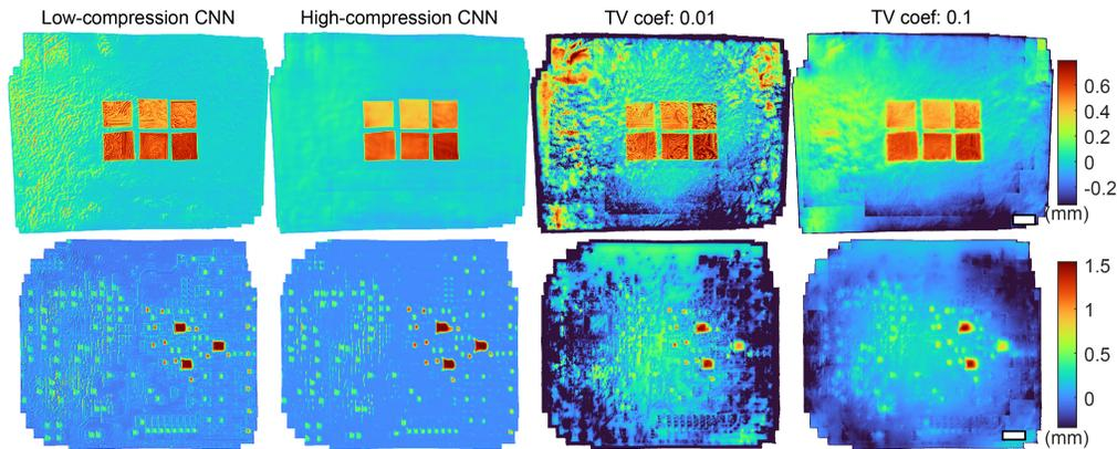
Figure 8. Height map reconstructions of the cut cards and PCB samples using high- and low-compression CNNs (architectures 1 and 4; see supplement for architectures and additional results) and high and low levels of total variation (TV) regularization. Zoom in to see fine features. Scale bars, 1 cm.
