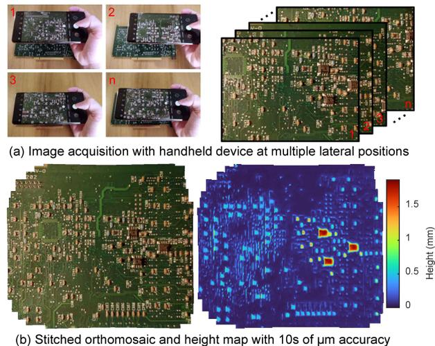
Figure 1. Our method jointly stitches multi-megapixel images acquired under freehand motion at close range and reconstructs high-accuracy height maps without precalibration of camera distortion.
