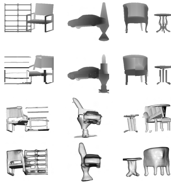
Figure 5. Comparison to a retrieval baseline which locally retrieves the nearest neighbors for depth patches of size N = 64 . First row: Test image. Second row: Image assembled from nearest neighbor patches from the training set. Third row: Reconstruction from the nearest neighbors (opposite viewpoint). Fourth row: Reconstruction from our Local@64 network.
