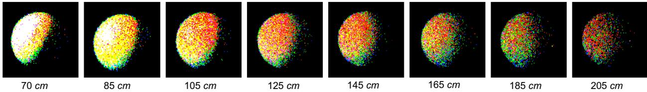
Figure 15. Examples of the relationship between distance of light source LED 0.5w and event streams(visualized based on the method in [2])
