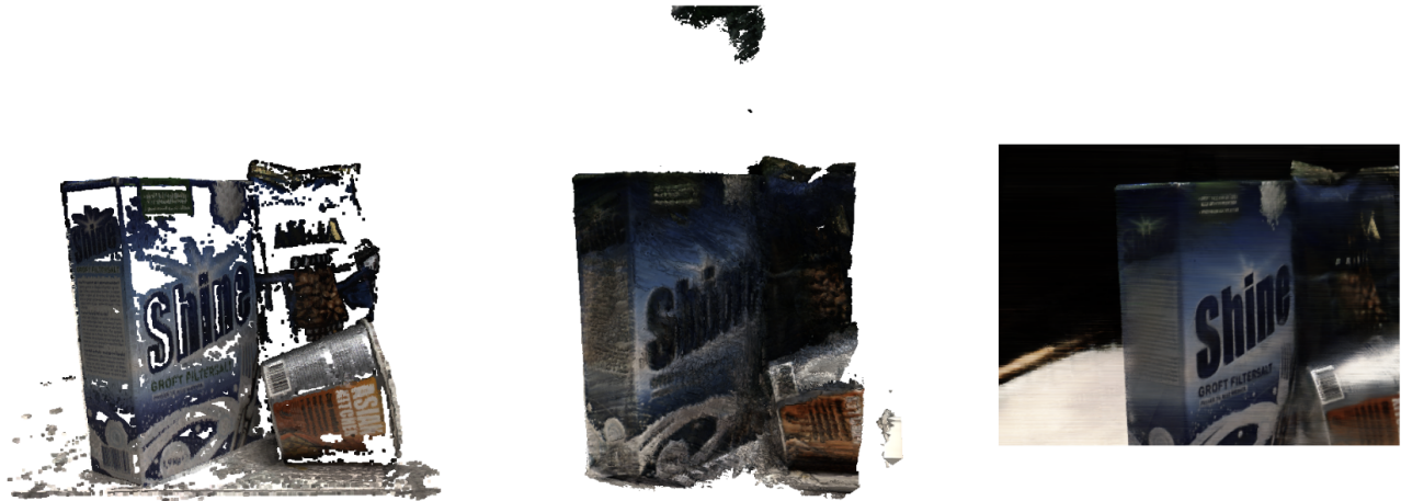
Figure 1. Left and middle: 3D reconstruction from 10 input images, obtained with COLMAP [5, 4] (left) and our SRF (middle). The COLMAP reconstruction is sharper but lacks complete surface, especially at uniform, textureless regions, see for example the characters of the logo “Shine”. 3D reconstruction of SRF can be more prone to noise (see top black spot) but is more complete. Right: Sharp novel view synthesised by SRF with full background.
