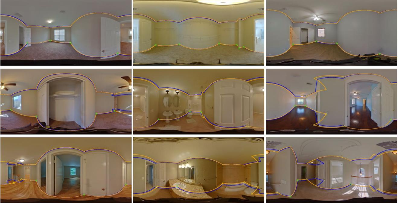
Figure 12: **Flat Ceiling:** Panoramas with flat ceilings in decreasing row order of F-score. The predicted layout is orange with corners denoted by triangles. The GT layout is in blue with corners denoted by crosses. Matched corners are highlighted in green.
