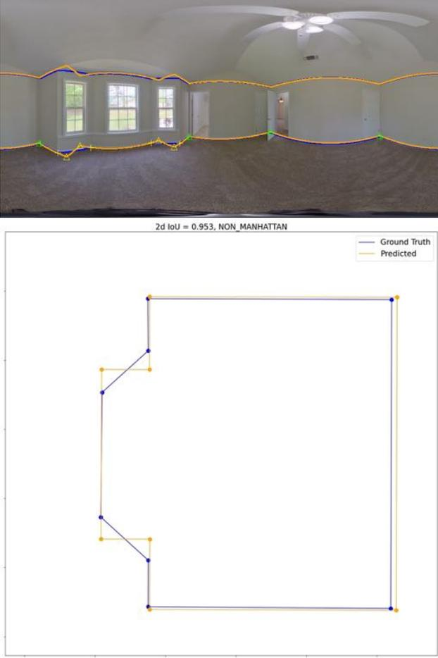
Figure 8: Shape with IoU > 95% despite failure to capture the structure of a bay window, requiring significant human touch-up. The Precision, Recall, and F-Score for **corner detection** all equal 50%.
