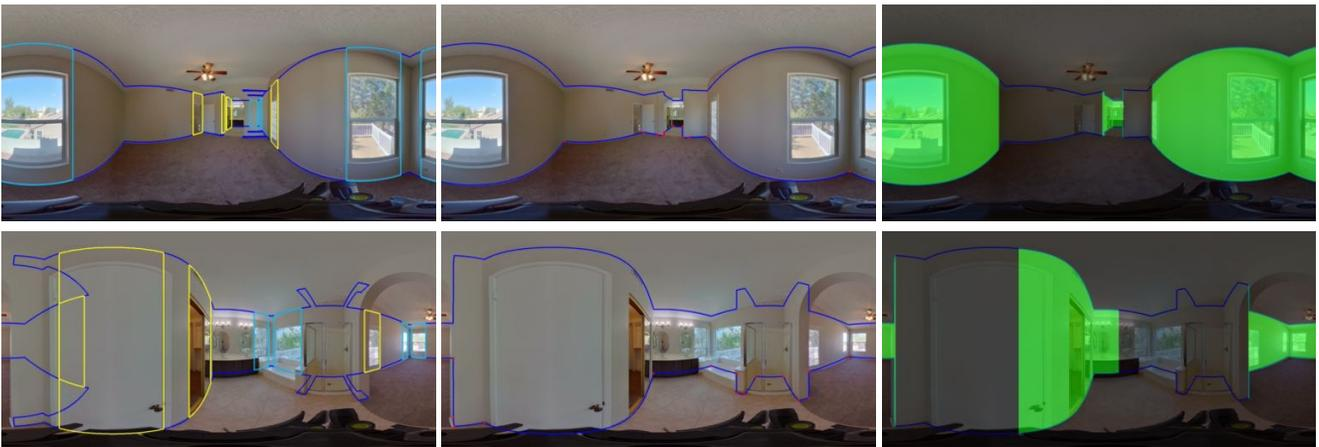
Figure 17: **Visible layout, covisibility map and covisibility score:** Examples of the derived visible layout, as well as the covisibility map and score calculation between pano pairs. We use ray casting to derive the visible layout polygon for each pano, as well as the covisibility map between pano pairs. In these two examples, the first pano pair has low covisibility, while the second pair has mid-range covisibility. The covisibility score is calculated as in section 6.2.
